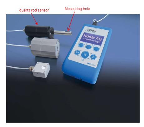
Measurement of UV intensity and dosage
